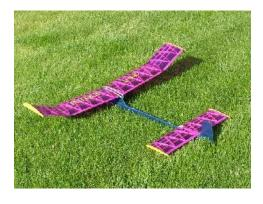
The plans show two rudder configurations. The one shown in these photos and a dorsal rudder ahead of the stab.
