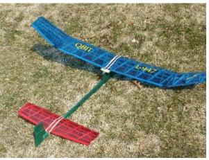
It has a pinch of right panel wash-in, but I don't think it's enough. If I use trailing edge stock, how much should be used and how thick?
